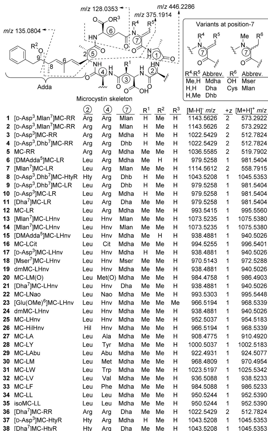
Fig. 1. Structures of MCs identified in the samples, and showing characteristic positive and negative mode fragments for MC-LR (12). Compound numbers in the text, Figures and Tables refer to the MC variants listed here. Compounds 13–26 and 35 do not appear to have been reported previously, and their tentative identities are based only on LC–HRMS/MS and chemical reactivity data. The positions of demethylation for some dmMC-LHnv variants could not be determined from the available data. Compounds 36–38 were only detected indirectly by mercaptoethanol derivatization, due to chromatographic overlap of the underivatized compounds with major isomer(s). An additional partly characterized variant with [M+H] + at m/z 972.5288 (25 + H 2 O) was also detected at 10.92 min (Table S3).
