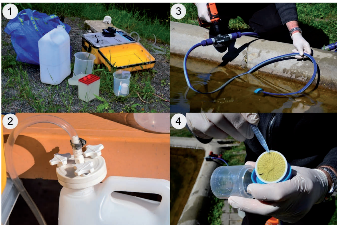
Figure 7: The two pump systems used during this PhD project. 1) The Masterflex portable peristaltic pump, 2) the in-line filter holder on top of a 5 L plastic can. 3) the drill-powered pump and 4) a filter being removed from the detachable filter-cups (4). Photos by Johannes C. Rusch.
