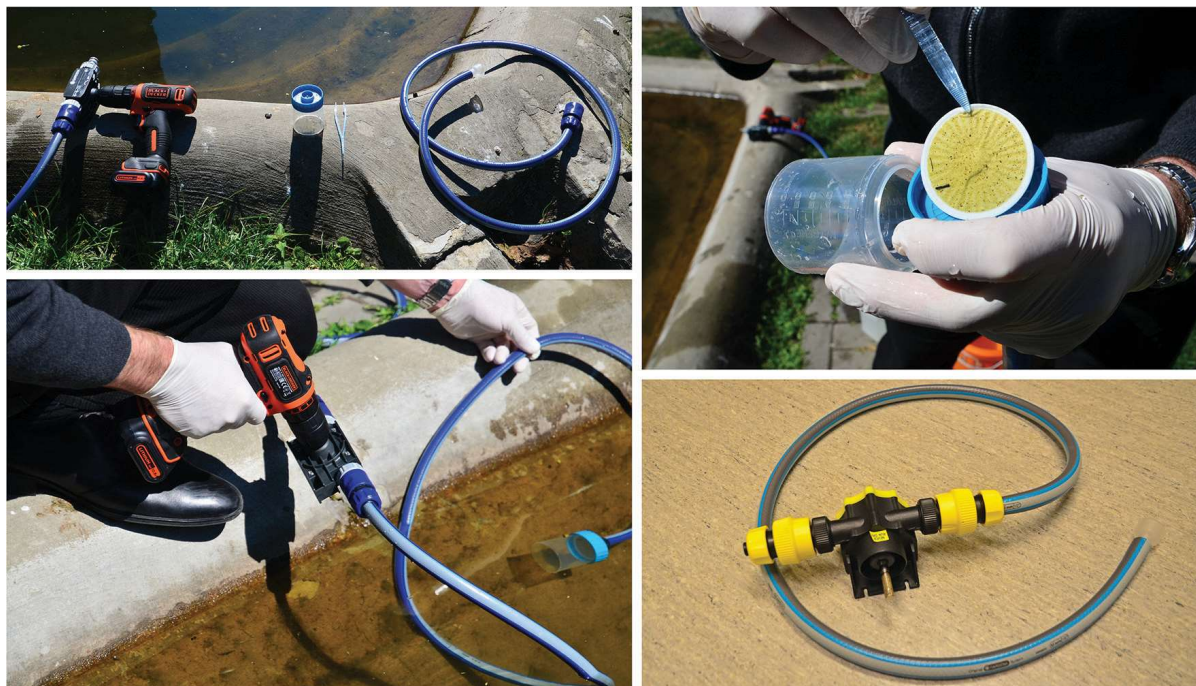
Figure 2. Drill-powered sampling equipment. The low-cost sampling equipment used in this study consisting of a drill-powered pump, single use forceps, filter cups and glass fibre filters. The pump depicted in the bottom right corner is one of many alternative models to the one used in this study.
