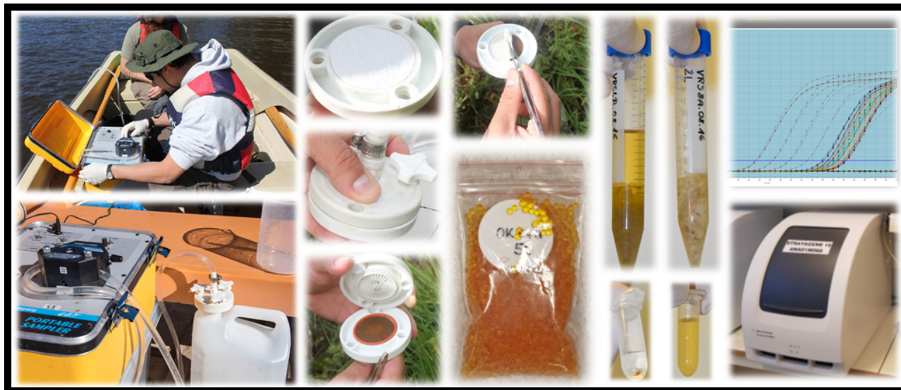
Figure 3. Water samples of ~5 L each were filtered on-site through glass fibre filters using a portable peristaltic pump (Masterflex E/S portable sampler). Each filter was carefully transferred to ziplock bag containing silica-gel beads for preservation until transportation to the laboratory. DNA was isolated with a large volume extraction procedure and presence/absence of eDNA from all target organisms was analysed using qPCR. Figure modified from Vrålstad et al (6).
