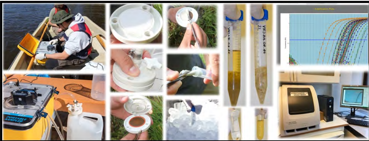
Figure 3. Water samples of ~5 L/ glass fiber filter were filtered on-site using a portable peristaltic pump (Masterflex E/S portable sampler). The filters were carefully transferred to a sterile falcon tube, stored on ice before being frozen in the laboratory. DNA was isolated with a large volume extraction procedure, and presence/absence of eDNA from all target organisms was analyzed with qPCR.
