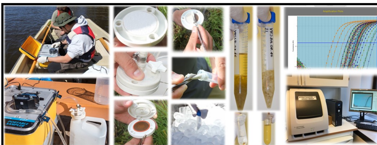
Figure 3. Water samples of ~5 L each were filtered on-site through glass fiber filters using a portable peristaltic pump (Masterflex E/S portable sampler). Each filter was carefully transferred to a sterile falcon tube, stored on ice before being frozen in the laboratory. DNA was isolated with a large volume extraction procedure, and presence/absence of eDNA from all target organisms was analysed with qPCR. Figure from Vrålstad et al (6).
